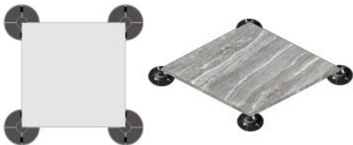
In the case of flooring for public use or where there are high loads, Florim recommends the adoption of additional supports under the slab, as in the diagram below
